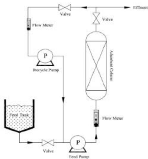
Fig. 1: Schematic diagram of experimental set up for the adsorption process
